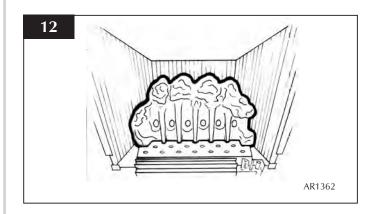
8.5 Place the front coal centrally in the channel at the front of the tray, Diagram 13. The relationship between the front coal and the flame baffle is shown in diagram 13.
